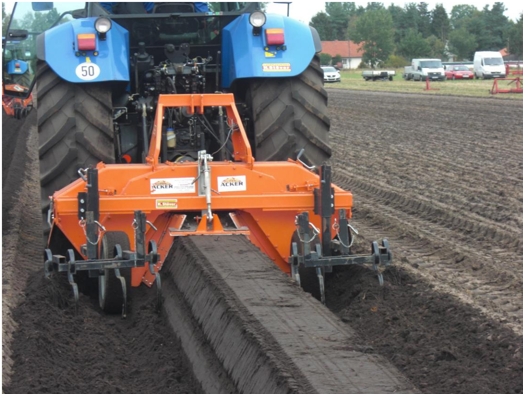
Making ridges for white asparagus cultivation
